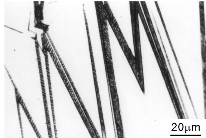
Thin plate (Fe-31Ni-0.23C, Ms=83K)
