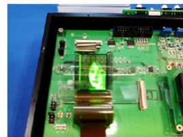
Scan-driver-integrated AM-OLED (LGE&ETRI, 2009)
