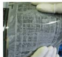
Flexible BW E-paper 5.35", VGA, 150ppi (Toppan, 2009)
