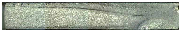
BM-A6061 ( \sigma_a=180\text{MPa} , N_f=2.6 \times 10^5 cycle)
