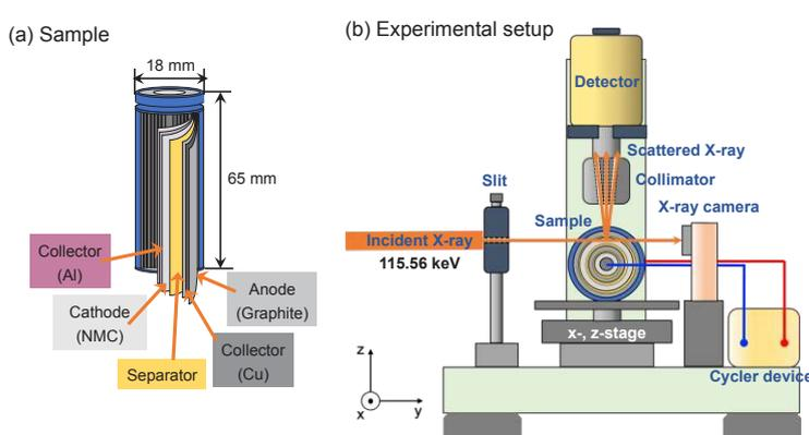
Fig. 1. Schematic image of the sample and experimental setup.
