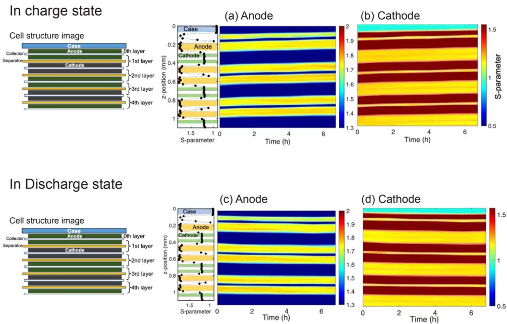
Fig. 3. (a) and (b) are S-parameter distribution of anode and cathode in charge state. (c) and (d) are S-parameter distribution of anode and cathode in discharge state.
