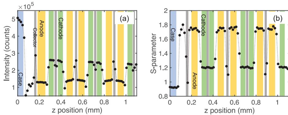
Fig. 2. (a) Compton scattered X-ray intensity and S-parameter
