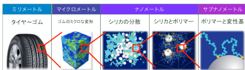
Figure 4. Multi-scale simulation consisting of large-scale FEM, MD and MO.
