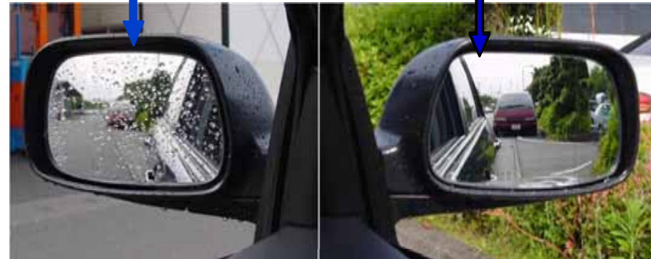
Fig. A mirror coated with a SiO 2 /TiO 2 multi-layered thin films is applied as such a side-mirror of cars.
