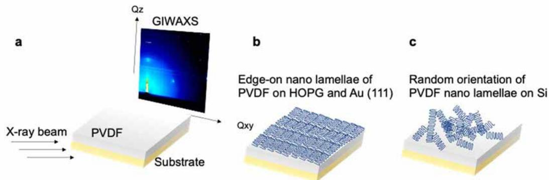
**Fig. 1:** (a) Schematics of the GIWAXS experiment where an X-ray beam grazes the substrate. The scattered X-rays are collected on a 2D detector placed behind the sample. (b) Schematics of 2~3 nm ultrathin PVDF nano lamellae arranged as edge-on lamellae on Au (111) substrate. (c) Schematics of 2~3 nm ultrathin PVDF lamellae arranged randomly on Si wafer.
