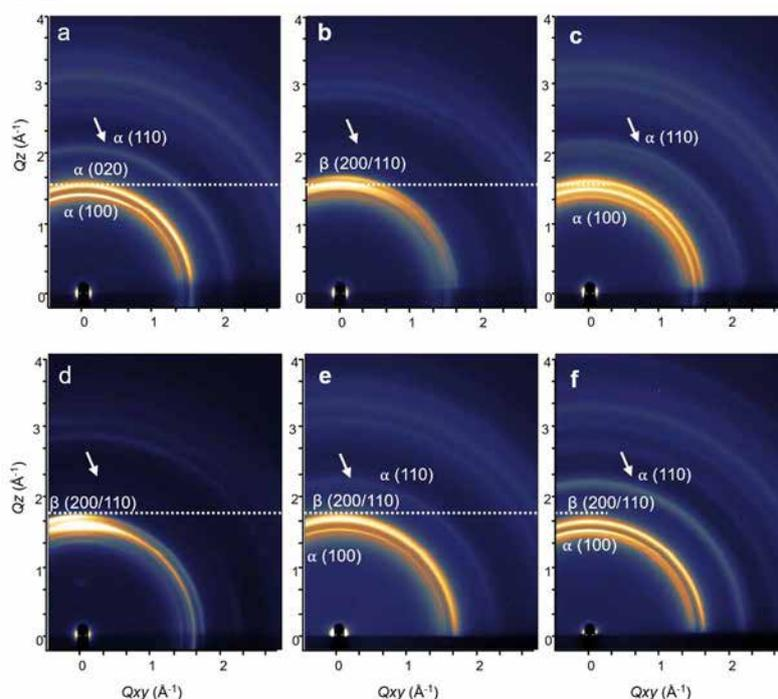
**Fig. 2:** GIWAXS pattern of ultrathin (a, b, c) pristine PVDF and (d, e, f) PVDF blended with GO placed on Si substrates under various stretching conditions. The white arrow in the figures indicates the  $\alpha$  (110). The white dotted line is drawn on all figures to distinguish the slight shift of the diffraction maxima for the  $\alpha$  and the  $\beta$  phases.
