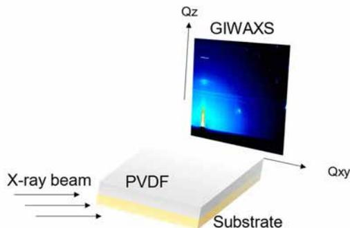
**Fig. 1:** Schematics of the GIWAXS experiment where an X-ray beam grazes the substrate. The scattered X-rays are collected on a 2D detector placed behind the sample.
