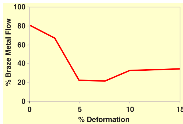
Fig. 2. Small amounts of cold work (3-5%) sharply reduce braze metal flow. More cold work brings some improvement [3].
