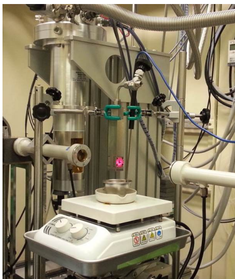
Fig.2. Image of in-situ Pd K-edge XAFS measurements by using an autoclave equipped with PEEK windows.
